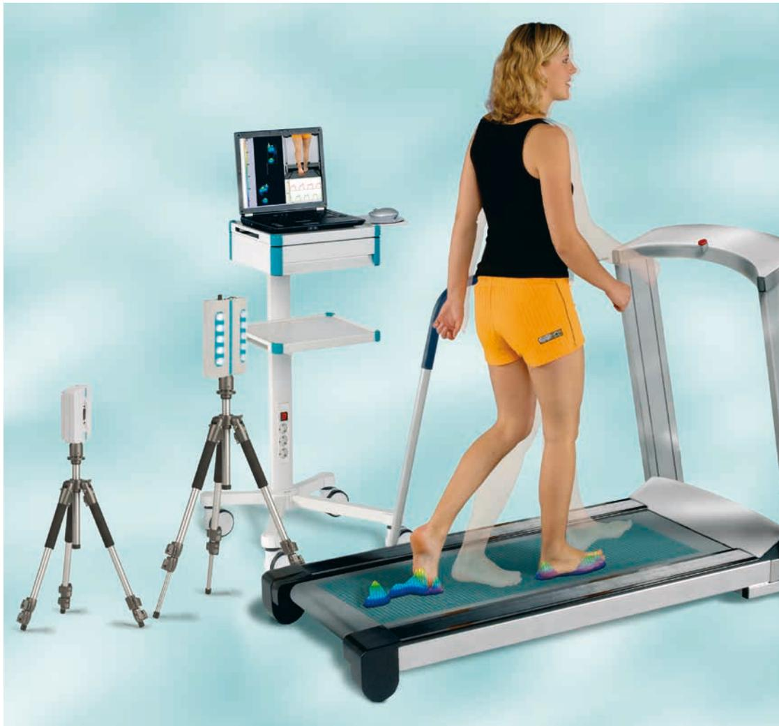
Using the zebris® FDM-T Analysis Center, gait and roll-off analyses can be carried out easily and quickly. The basic system can be extended in a variety of ways with video, motion analysis and EMG.
