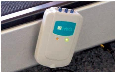
The infrared synchronization adapter is connected to the junction box of the treadmill ergometer.
