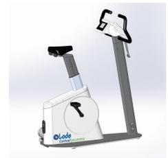
Eccentric ergometry or “negative ergometry” is used to train severe pulmonary and cardiac patients. The motor is pushing the crank axle of the ergometer in the opposite direction. The test subject has to resist this workload and keep the pedal frequency at a selected number to get the desired training effect.
